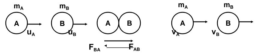
If two balls A and B of masses  $m_A$  and  $m_B$  are travelling in a straight line with initial velocities  $u_A$  and  $u_B$  and if  $u_A > u_B$ , the two balls will collide with each other. During collision at a time t, ball A exerts a force  $F_{AB}$  on ball B and ball B exerts a force  $F_{BA}$  on ball A. If  $v_A$  and  $v_B$  are the velocities of balls A and B after collision,
